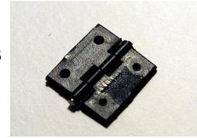
Be very careful when using glue near pinned part of the hinge. First insert the hinge into hinge hole and then apply the glue from inner side of the wing. Do the same when gluing aileron to hinge. First insert all hinges into hinge holes on aileron and then apply glue from inner side of aileron. Make sure that aileron has enough space for moving from every side.
