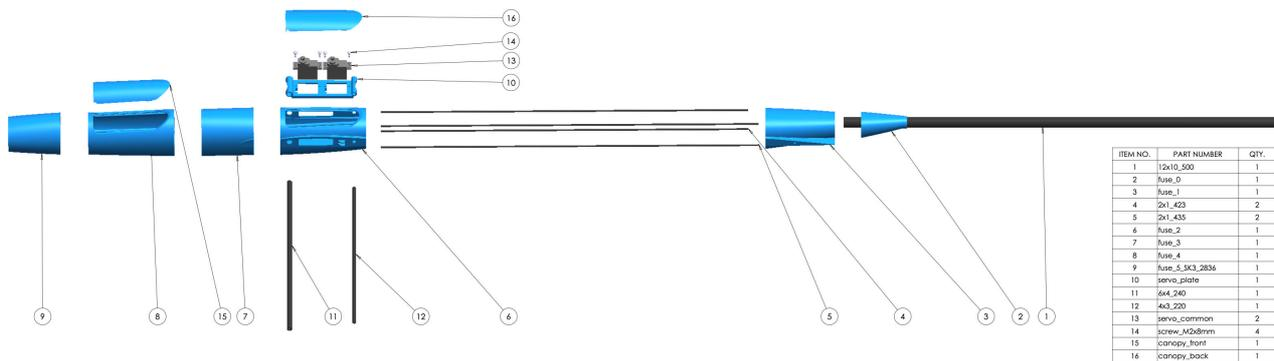
Start by gluing together boom and fuse\_0. Boom should protrude 2cm from the fuse\_0 part. When these two parts are aligned correctly apply glue from the tail side of the wing. fuse\_0 part has tiny channels for glue to soak in along the boom.
