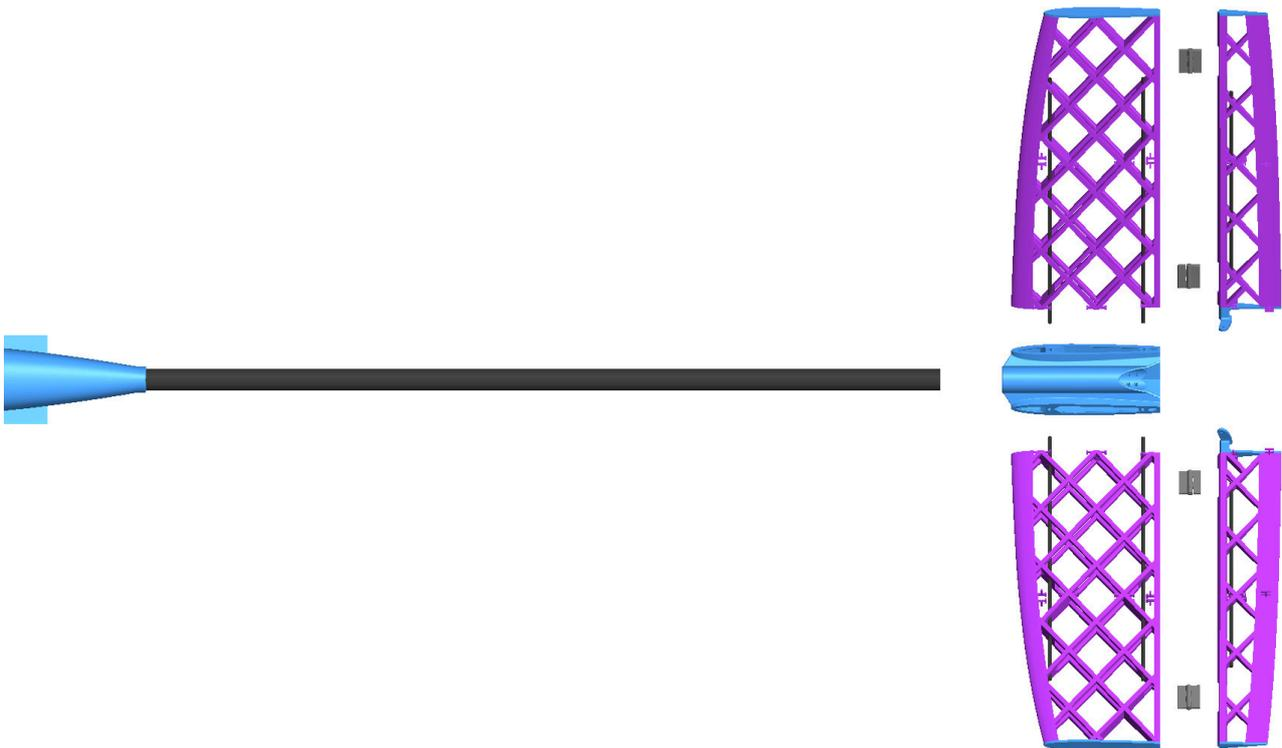
To complete tail assembly first shorten all hinges and then insert the hinges into hinge slots and apply the glue from inner side of the main tail. Then insert all hinges into hinge slots on moving part of the tail and put the glue from inner side of the moving part. Tip of the moving part should be aligned flush with main part.
