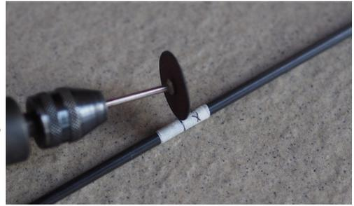
TIP: Carbon wing joiner tubes on the fuselage should fit into spars in the wing. Sometimes the fit is too tight or you cannot insert joiner tubes into wing spars at all. You can use drill and wet sandpaper to make joiner tubes thinner. Use breathing mask to avoid inhaling carbon dust!
