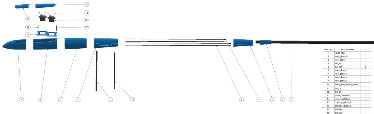
Start by gluing together boom and fuse\_glider\_0. Boom should protrude 2 cm from the fuse\_glider\_0 part. When these two parts are aligned correctly apply glue from the tail side of the wing. fuse\_glider\_0 part has tiny channels for glue to soak in along the boom.
