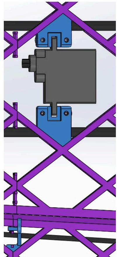
forget to center your servos before gluing them in. Check also that servo arm holes fit your clevises and enlarge the holes if necessary, drilling them when servo is in place could damage the wing.
