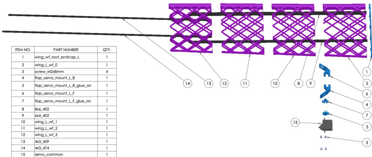
Wing with flaps has the same parts as the aileron only wing, except for the first 4 sections and wing alignment spar. That is why the drawing shows only half of the wing, the rest should be assembled exactly same as already described above in *Wing (without flap option)* section starting with aileron servo mount and wing\_L\_4. Main carbon spars (8x6\_402 and 6x4\_402) should be aligned flush with base of wing\_wf\_root\_endcap\_L part.
