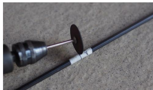
TIP: Joiner rods on the fuselage have diameter of 4 mm, carbon spars in wings have inner diameter of 4 mm. They should fit into each other but sometimes the fit is too tight or you cannot insert joiners rods into wing spars at all. You can use drill and wet sandpaper to make joiner rods thinner. Use breathing mask to avoid inhaling carbon dust!
