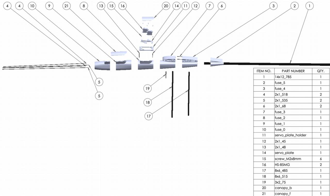
Start by gluing together boom and fuse\_5. Boom should protrude 4 cm from the fuse\_5 part. Apply glue from the tail side of the wing. fuse\_5 part has tiny channels for glue to soak in along the boom.
