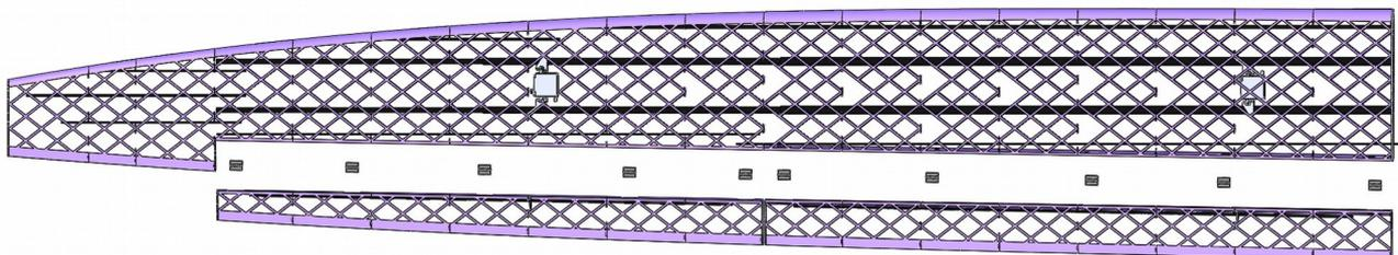
To complete wing assembly attach aileron and flap to the wing.
