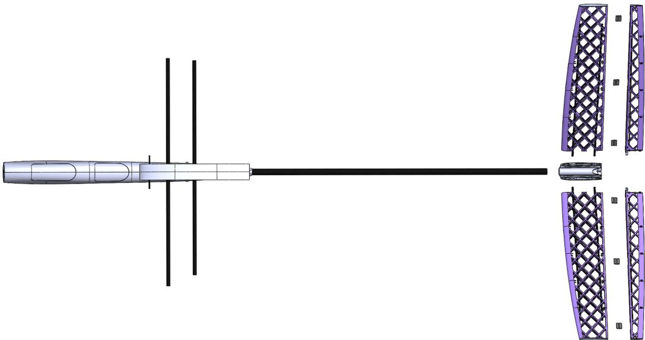
To complete tail assembly first shorten all hinges and then insert the hinges into hinge slots and apply the glue from inner side of the main tail. Then insert all hinges into hinge slots on moving part of the tail and put the glue from inner side of the moving part. Tip of the moving part should be aligned flush with main part. Be very careful when using glue near pinned part of the hinge.
