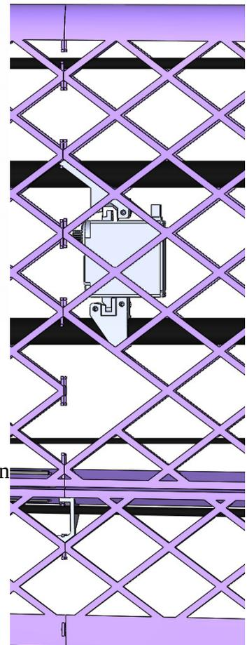
Assembly first section of left wing as sketched above. Main spars (10x8\_745) and front alignment spar (4x3\_985) should be aligned flush with base of wing\_root\_endcap\_L part. Rear alignment spar (2x1\_809) should protrude 1 cm from wing\_root\_endcap\_L part.
