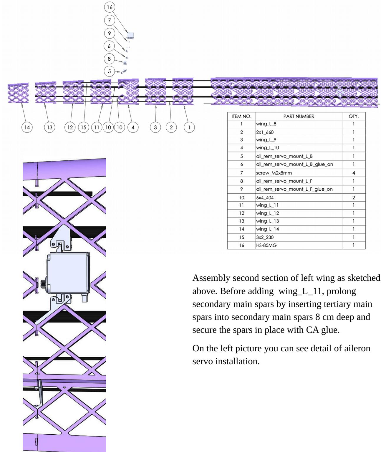
Assembly second section of left wing as sketched above. Before adding wing\_L\_11, prolong secondary main spars by inserting tertiary main spars into secondary main spars 8 cm deep and secure the spars in place with CA glue.
