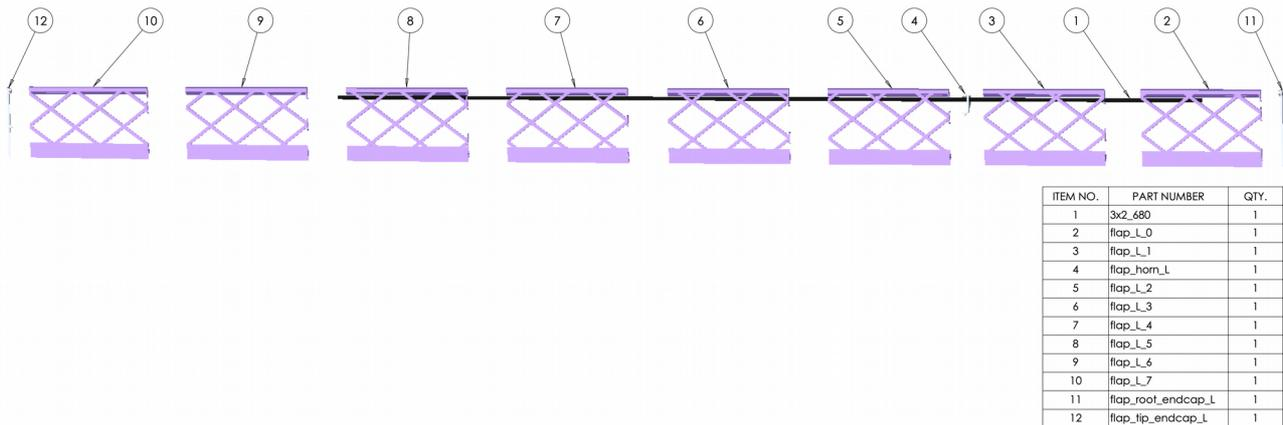
Assembly left flap as sketched above. Don't forget to insert flap\_horn\_L part between flap\_L\_1 and flap\_L\_2. Flap horn should stick out from the bottom side of the wing. When all the parts are in their position, put glue on contact points where carbon spars are touching printed parts. Put also a bit of glue on trailing edge where all the flap sections are touching each other.
