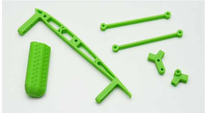
2. Shell parts (wings). Use 0% infill and no horizontal surfaces (thickness of the shell is one layer). Only this way you can achieve required weight of the plane.
